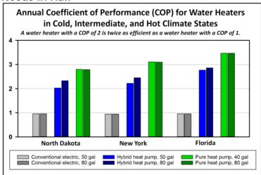
The National Resources Defense Council conducted a new study that shows water heaters using high efficiency heat pump technology can cut electricity needs to heat water by at least half. Considering heating water accounts for about 13% of total residential energy use, the impact are far reaching.
